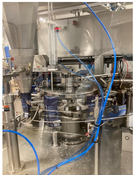
Step 2 Gas injection station
