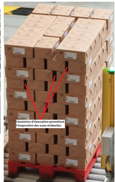
Finalized pallet of 5 boxes where the ducts are visible.
