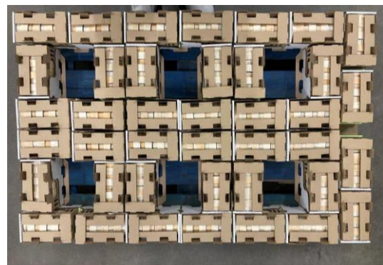
Pallet with its “ducts” seen from above
